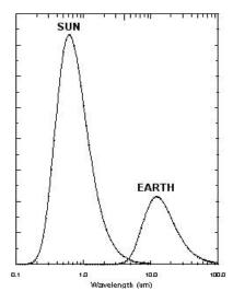
This diagram plots the relative intensity of the black body radiation from the sun and the earth as a function of wavelength.
